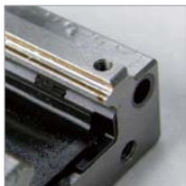
Inspection point 1 and 2 : Lubrication result
