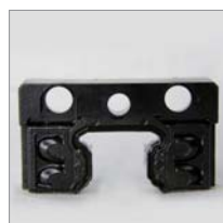
End seal in good condition
