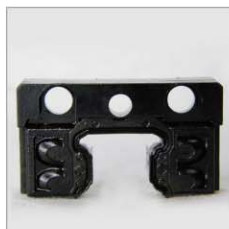
End seal in good condition
