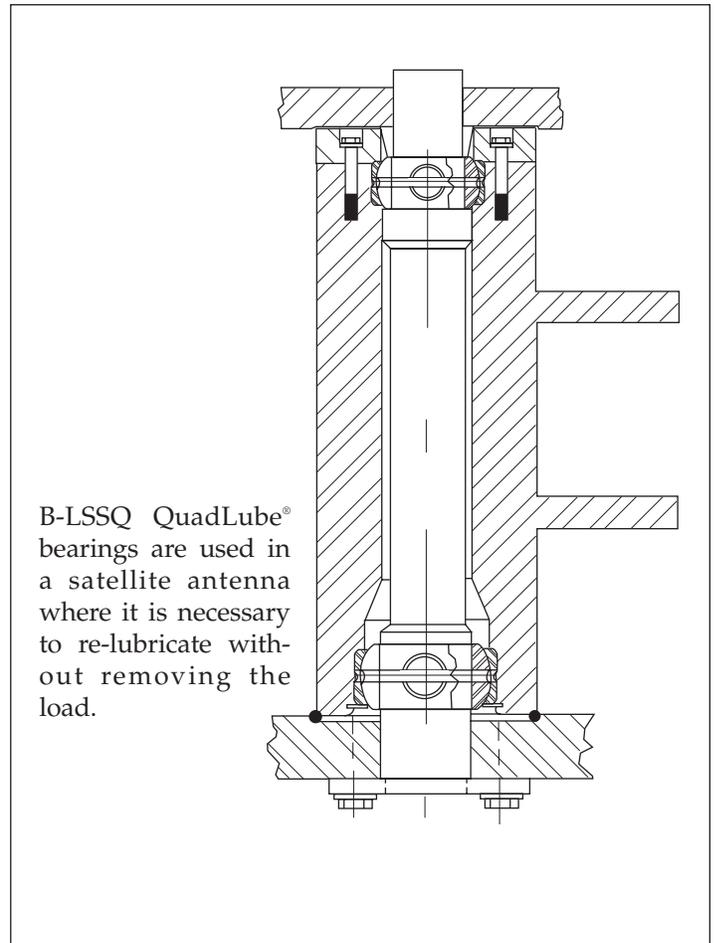
B-LSSQ QuadLube® bearings are used in a satellite antenna where it is necessary to re-lubricate without removing the load.
