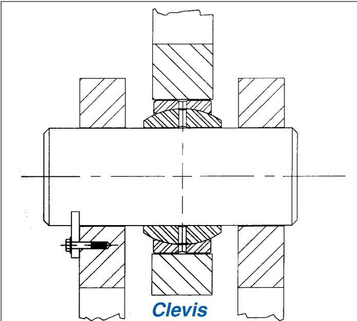
The boom cylinders and connections on the shovel incorporate a B-L bearing into a typical clevis mount application.
