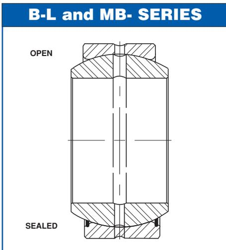
Designed to support heavy radial loads under misalignment. These bearings also possess moderate thrust loading capability. They are non-separable with a single fractured outer ring, and are available in open or sealed designs and inch or metric sizes.
