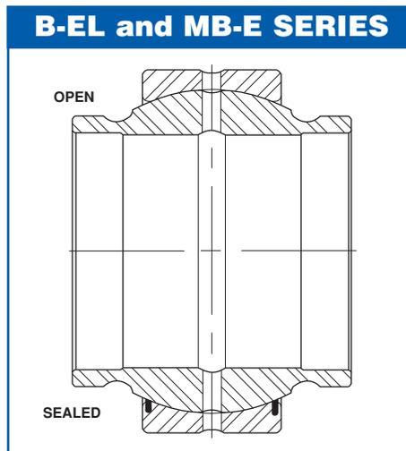
With an extended inner ring, the need for additional locational spacers is eliminated. The inner ring bore is relieved to prevent excess bending stress. Available in open or sealed designs and inch or metric sizes.
