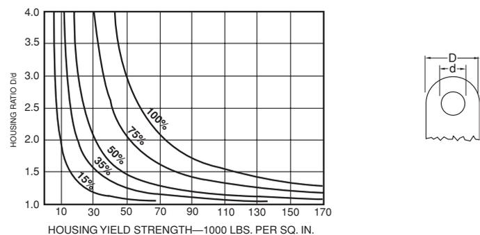
Figure 17: Influence of Housing Design on Bearing Capacity
