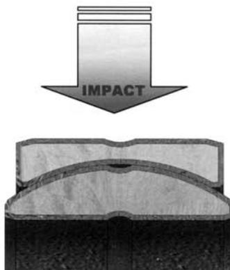
Innovative hole and notch designs facilitate fracturing of the ImpactTuff® Outer Ring for bearing assembly
