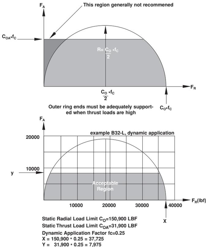
Figure 13: Radial Bearings
