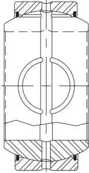
Up to 300% improved service life provided by innovative lubrication system. The patented system distributes lubrication to the load zone even when no load reversal exists and allows re-lubrication without removing the load. These bearings provide an increased life to many problem applications. Available in inch or metric sizes.
