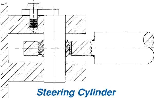
The steering cylinder of the loader uses a B-L bearing where radial loads are present.
