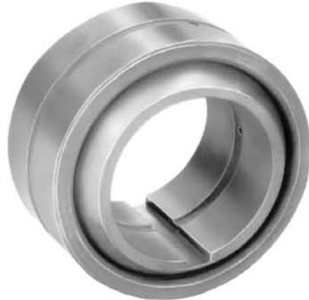
An extended inner ring spherical plain bearing with spiral lubrication grooves in the bore of the inner ring to facilitate lubrication flow. This bearing is used in the suspension of a heavy duty industrial trailer.
