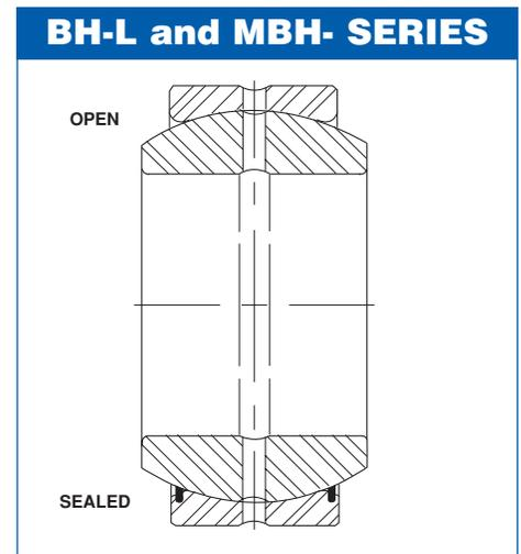
Due to greater inner ring cross section, the BH-L and MBH series is capable of greater misalignment. Available in open or sealed designs and inch or metric sizes.
