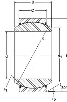
RBC's DuraLube™ self-lubricating spherical plain bearings provide long life in demanding applications. Grease-free operation is accomplished through the use of a durable PTFE liner system that reduces friction between the spherical surfaces of the inner ring and outer ring. These bearings are ideal for applications in which re-lubrication is impractical or impossible, but longevity is a must. Available in inch or metric sizes.
