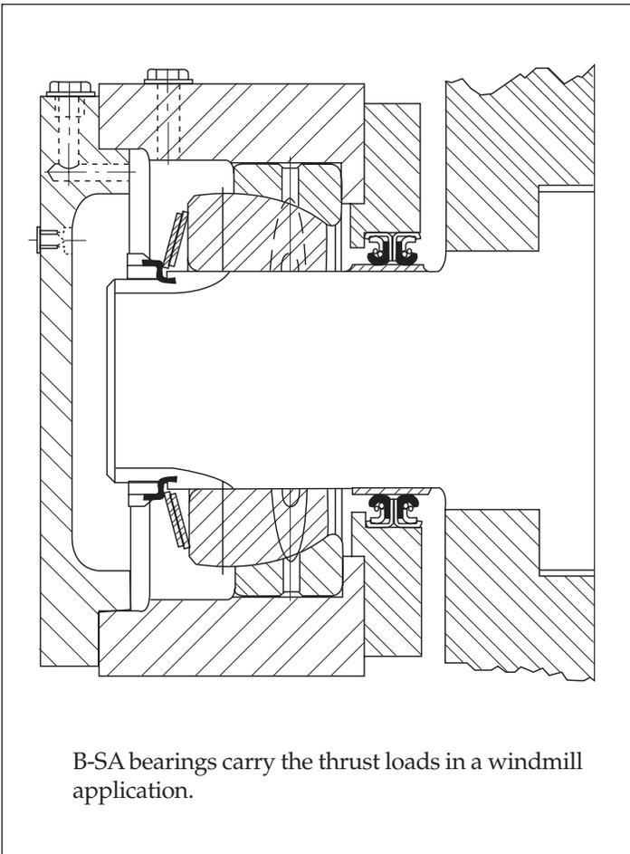
B-SA bearings carry the thrust loads in a windmill application.
