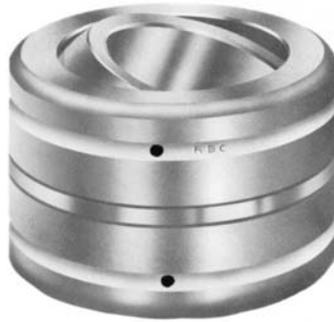
The RBC ShimPack® double acting angular contact spherical plain bearing was developed to ease the installation procedures required on the assembly line. Traditionally the bearing assembly was completed, clearance was measured and then the assembly was disassembled, shimmed and reassembled. With the RBC ShimPack® double acting angular contact spherical plain bearing, a spacer is preset and individually calibrated at the factory to provide the optimum amount of axial internal clearance.
