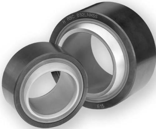
RBC's DuraLube™ self-lubricating spherical plain bearings provide long life in demanding applications. Grease-free operation is accomplished through the use of a durable PTFE liner system that reduces friction between the spherical surfaces of the inner ring and outer ring. This proprietary liner system has been developed for rigorous industrial applications, and has been proven successful time and time again.
