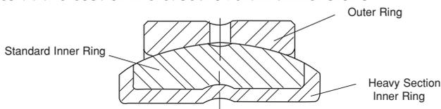
**Figure 5: Standard vs. Heavy Section Inner Ring**
