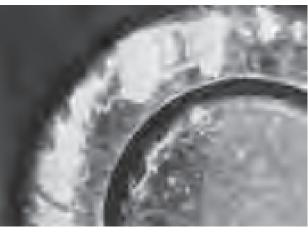
Fig. 15-4 Scratches on Larger Side Surface of Tapered Roller Bearing
