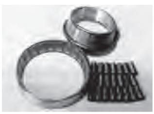
Fig. 15-12 Corrosion on Tapered Roller Bearing
