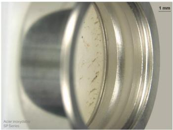
The results of the salt spray test confirm that SP-grade steel has superior corrosion resistance, with no evidence of corrosion compared to the high-corroded 440C stainless steel.
