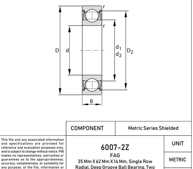
Radial, Deep Groove Ball Bearing, Two **Metal Shields**
