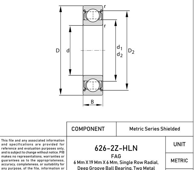
Deep Groove Ball Bearing, Two Metal Shields
