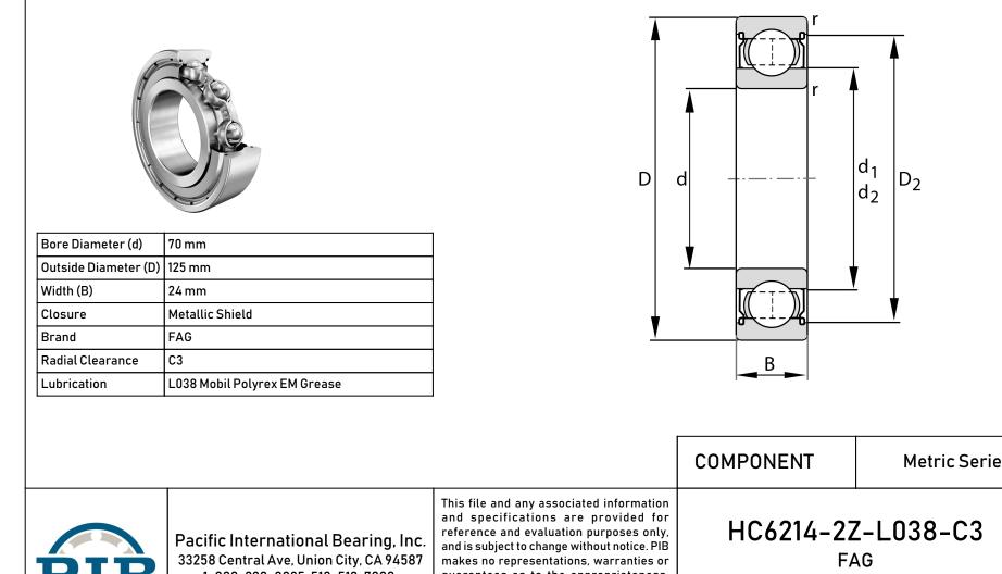
**Metric Series Shielded** UNIT METRIC guarantees as to the appropriateness, 1-800-228-8895, 510-512-7000, Fag, 70 Mm X 125 Mm X 24 Mm, Single Row accuracy, completeness, or suitability for info@pibsales.com Radial, Deep Groove Ball Bearing, Two any purpose, of the file, information or www.pibsales.com specifications. You are solely responsible **Metal Shields** SHEET for the use of the file, information or specifications.
