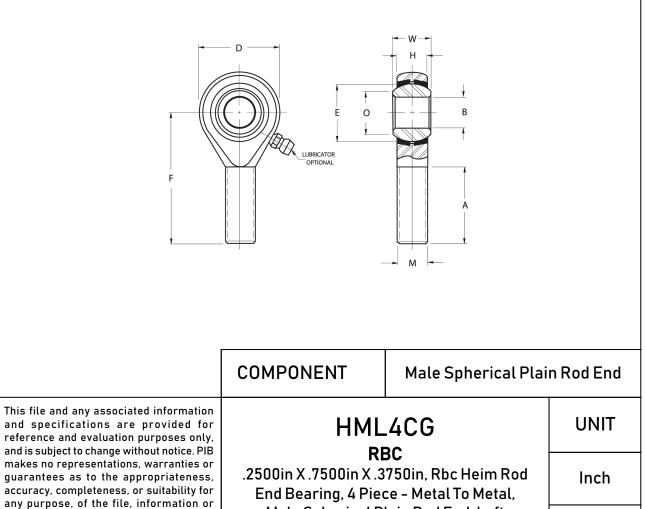
Male Spherical Plain Rod End, Left Handed Thread SHEET
